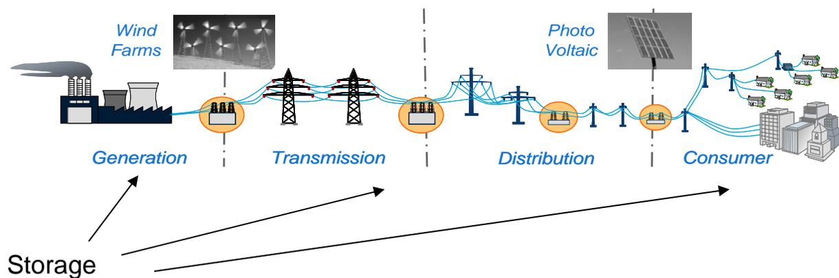
Energy storage is not new. Pumped-hydro systems and lead-acid batteries have been in operation for many years and the concept of Compressed Air Energy Storage (CAES) has been known for many years as well. Newer technologies that are in the early market adoption stages, such as lithium ion batteries, flow batteries, flywheel, and sodium sulphur (NaS) systems offer improved operational flexibility, and in some cases longer duration or fast response capabilities.
